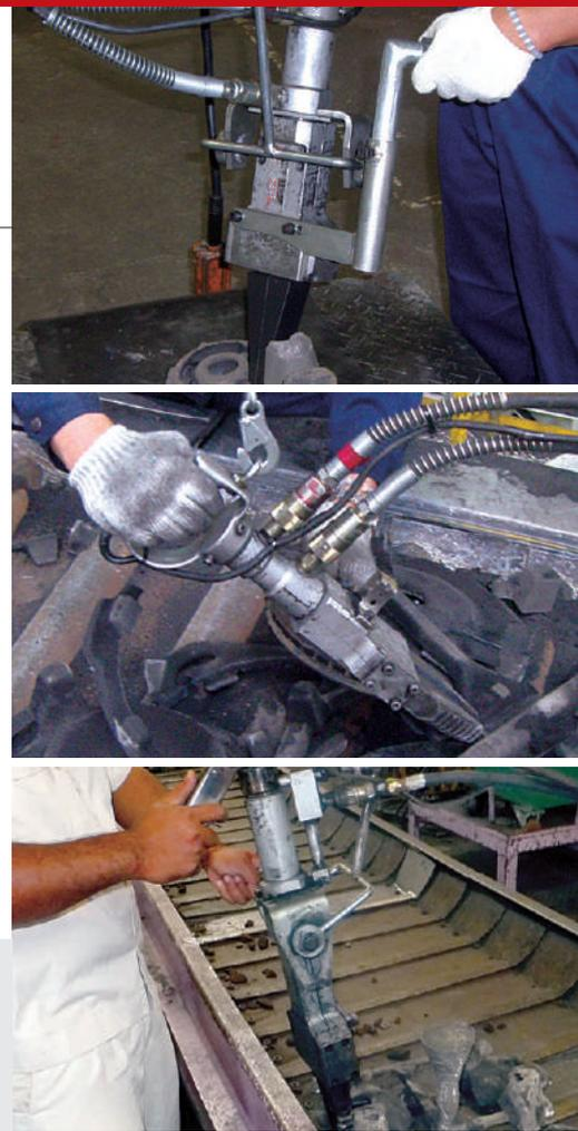
The Casting Splitter EP-Series, for splitting gates from iron castings. Compared to traditional hammering, plasma cutting and grinding methods, the EP-Series provide easier, faster and safer solutions.
