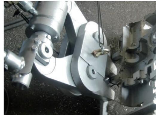
The Metal Cutter Series are specially designed to cut risers and feeds of non-ferrous materials such as aluminium, bronze and copper. Both models use specially developed and hardened blades to cut through the material without bending or damaging them. Operation is fast, easy and with the simple click of a button. All models are manually operated machines, but can be adapted for online systems.
